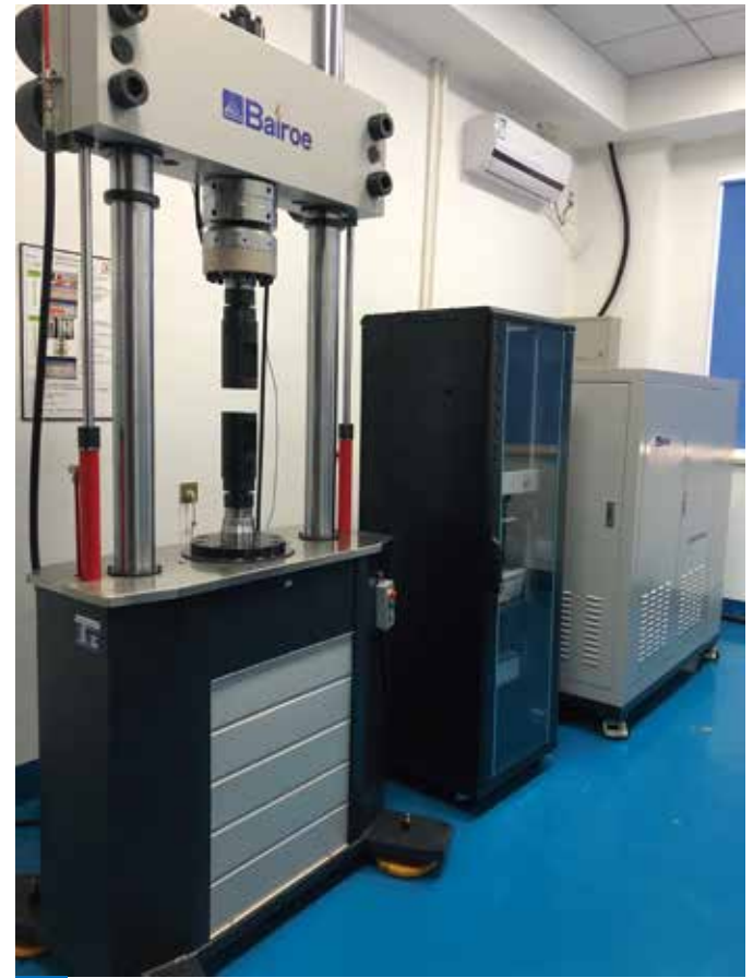
微电脑控制液压伺服疲劳试验机 主要对金属和非金属材料进行轴向对称性循环疲劳试验 Microcomputer Control Hydraulic Servo Fatigue Testing Machine for Tension Test -- Axial symmetry cyclic fatigue test for metallic & non-metallic materials
