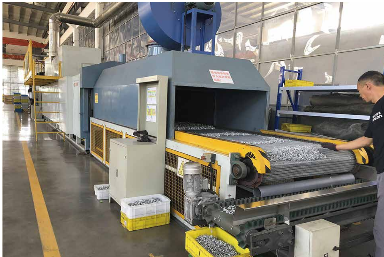
达克罗涂层工艺生产线，比电镀锌更耐腐蚀性，并可通过盐雾试验约500-1000小时。 Dacromet Production Line ,Make The Fasteners Which Coating Dacromet Stronger Corrosion Resistance Than Zinc Plated Or Galvanized, and Can Pass Salt Spray Test About 500 to 1000 Hours .
