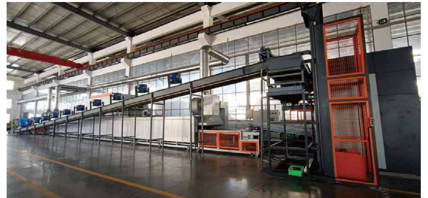
龙门可倾式浸甩达克罗涂覆生产线 Gantry tilting dipping Dacromet coating production line
