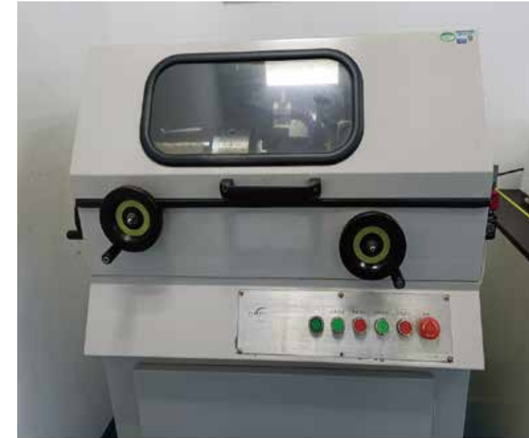
试样切割机 Sample cutting machine
