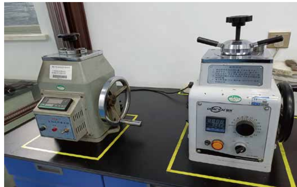
金相试样镶嵌机 Metallographic specimen mosaic machine
