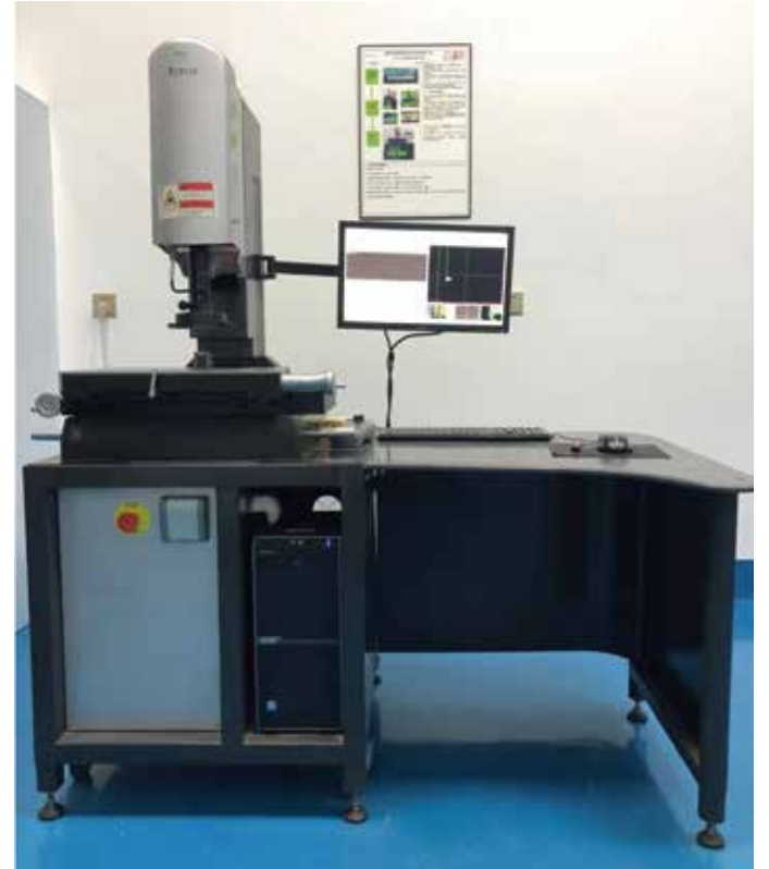
影像测量仪 测量点、线、圆、弧、椭圆、矩形，提高测量精度 Video Measuring Instrument -- Measure points, lines, circles, arcs, ellipses, and rectangles to improve measurement accuracy
