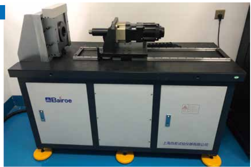
紧固件横向振动试验机 Fastener Transverse Vibration Test Machine It can inspect the fastener self-locking performance (the anti-loosening performance) under the certain frequency and amplitude transverse dynamic loading.
