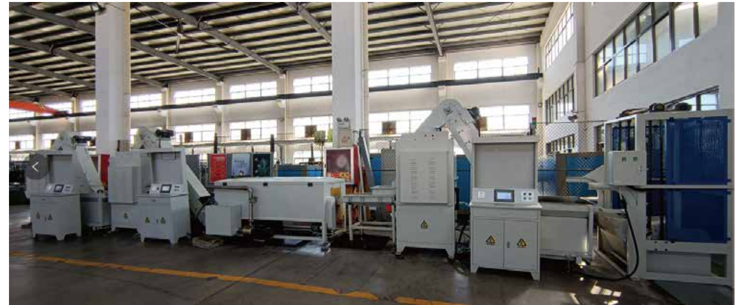
产品本色涂油防锈自动生产线 Automatic production line for oil coating and rust prevention
