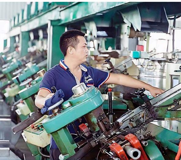
Through a manufacturing process including heading, wire drawing, annealing, threading, heat treatment, electroplating, washer assembling, packaging and shipping, Honghui provides clients with one-stop fastener service. It can also design and manufacture various self-drilling and self-tapping screws per clients’ requests. Currently it can manufacture up to more than 20,000 tons of high quality carbon steel and stainless steel self-drilling screws annually.
