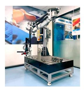
In addition, when coupled with ultrasonic equipment, the simulated assembly system can also obtain fastening parameters such as torque, angle, axis force, coefficient of friction, coefficient of torque, and a variety of assembly parameter curves of the threaded connection during the fastening process, which is conducive to a more detailed analysis of threaded connection.
