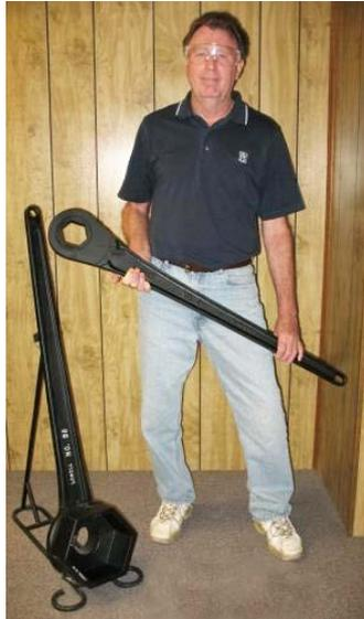
The cast malleable iron 40 Series wrenches are available up to 48" long with square, hex, or round/keyed openings up to 4-1/2". They include reversing controls in the head and enclosed replaceable gears. Additionally, the tools' Bolt-Thru design makes it easy to tighten nuts on any threaded length. Above all, Lowell designs its extra-large wrenches to be safe, accessible, and customizable to your needs.
