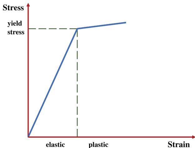
Figure Two Stress/Strain Graph for a Material in Tension
