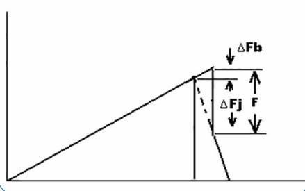
If the bolt is less stiff, with respect to the joint, the bolt will experience a smaller percentage of the external load, which depends upon the stiffness ratio of the bolt and joint. This helps in
