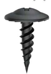
UFO modified round head design provides a flat finish on the steel surface and ensures a tight fit. The 15% deeper Phillips recess provides higher torque resistance and minimizes camming out. The patented G2 point can easily penetrate steel up to 20GA+20GA, making it a superior replacement for conventional fasteners.
