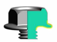
the neck to the outer periphery, and a continuous undercut section located at the outermost periphery. It has a cup shape consisting of a flat part. When fastened, this part elastically deforms and acts like a spring washer, so you can get a strong locking effect without using a spring washer or flat washer. Additionally, by reducing the number of parts, the Cup Bolt achieves a weight reduction of approximately 18% compared to conventional models.
